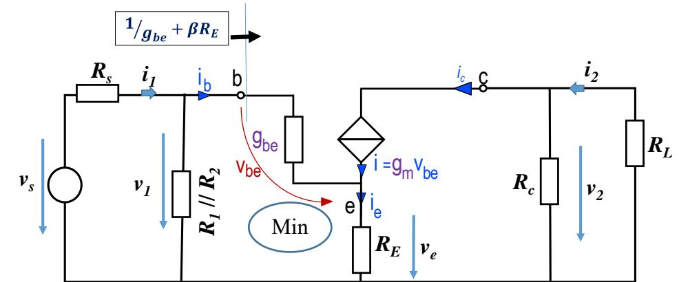
$$\bullet \quad A_v = \frac{v_2}{v_1} = \frac{-i_c (R_c // R_L)}{i_b (1/g_{be} + \beta R_E)} = \frac{-\beta (R_c // R_L)}{(1/g_{be} + \beta R_E)} \approx \frac{-R_c // R_L}{R_E}$$
