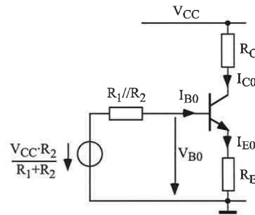
$$V_{CC} \cdot \frac{R_2}{R_1+R_2} = (R_1//R_2) \cdot I_{B0} + U_j + R_E \cdot I_{E0} = (R_1//R_2) \cdot \frac{I_{C0}}{\beta} + U_j + R_E \cdot I_{C0}$$
